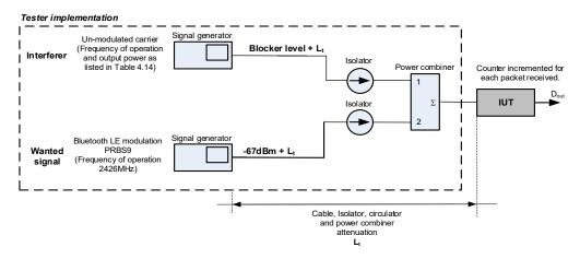
Figure 4.22: Blocking performance test setup
