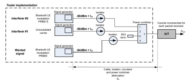
Figure 4.23: Test setup for intermodulation test
