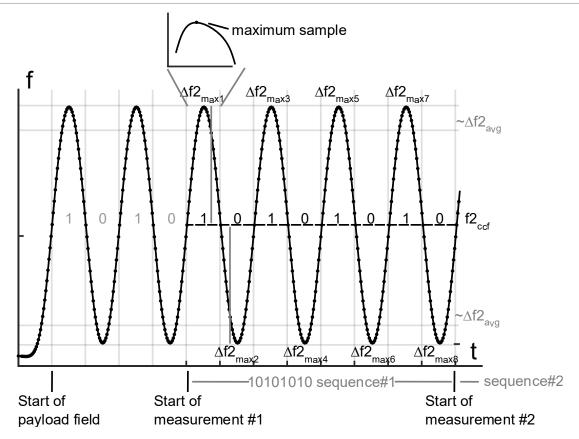
Figure 4.6: Frequency deviation measurement principle for 10101010-payload sequence
