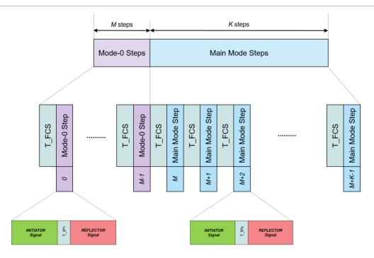
Figure 4.4: Channel Sounding RFPHY test signal transmission overview
