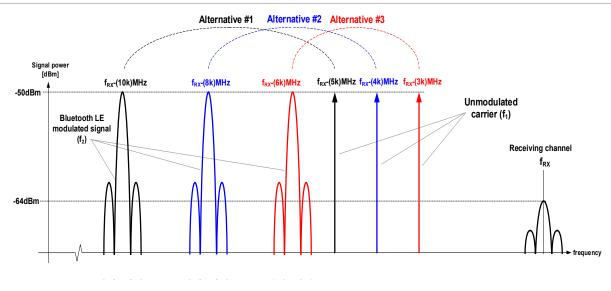
Figure 4.24: Test signal allocation alternatives in the frequency domain at symbol rate k (in Ms/s). Note: figure shows only frequencies below fo.
