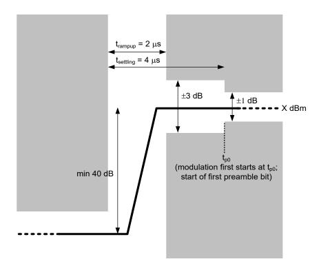
Figure 6.1: Lower Tester ramp-up characteristics requirement, modulation first starts at tpo
