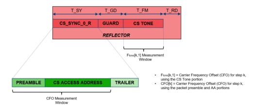
Figure 4.25: Step Mode-0, Reflector signal CFO measurement windows
