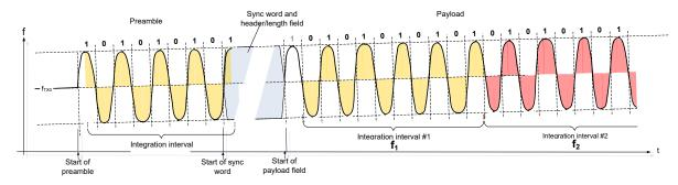
Figure 4.8: Frequency drift measurement principle
