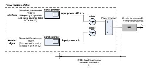
Figure 4.21: C/I and receiver selectivity test setup
