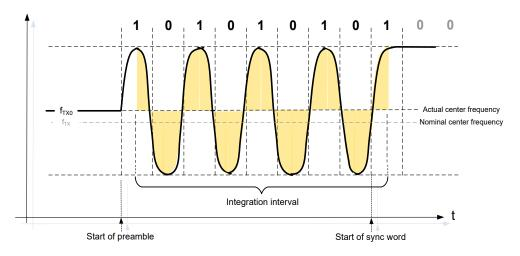
Figure 4.12: Initial carrier frequency (f<sub>0</sub>) measurement principle for 1 Ms/s
