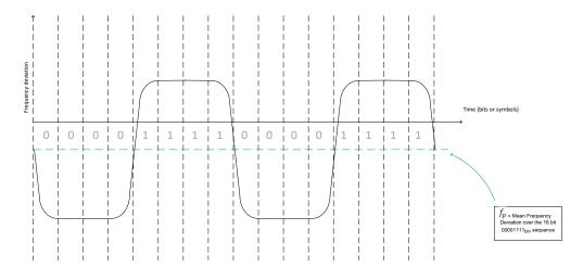
Figure 4.14: Average center frequency measurement (fp) principle
