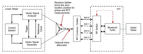
Figure 4.3: Test Equipment Setup for Channel Sounding
