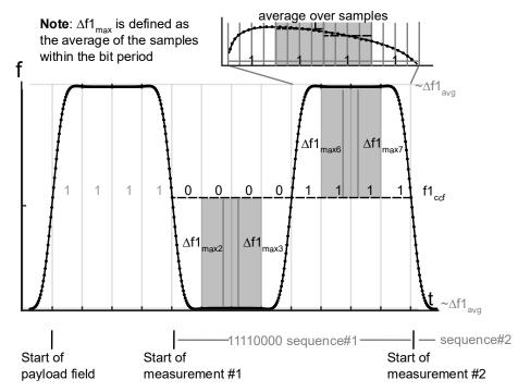
Figure 4.11: Frequency deviation measurement principle for 11110000-payload sequence
