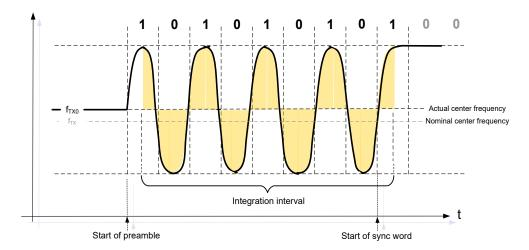
Figure 4.7: Initial frequency offset (f<sub>0</sub>) measurement principle
