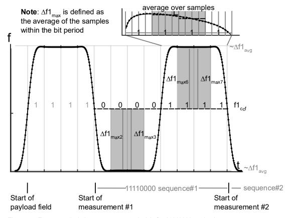
Figure 4.5: Frequency deviation measurement principle for 11110000-payload sequence
