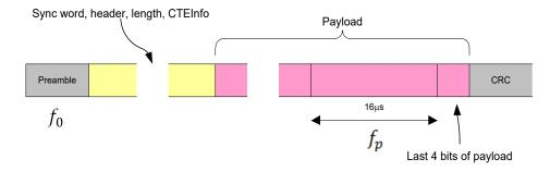
Figure 4.13: Average center frequency measurement (fp) measurement location
