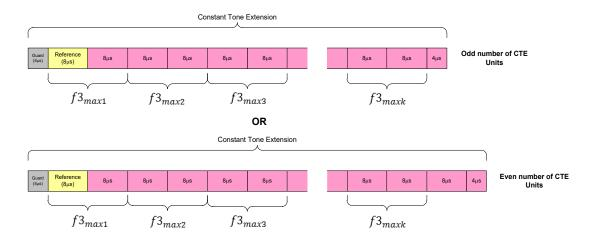
Figure 4.15: Average frequency deviation measurement principle
