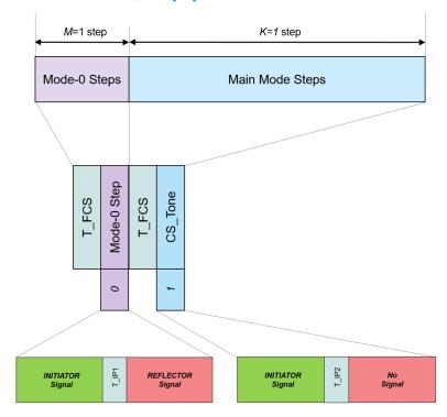
Figure 4.16: Stable Phase test signal transmission overview
