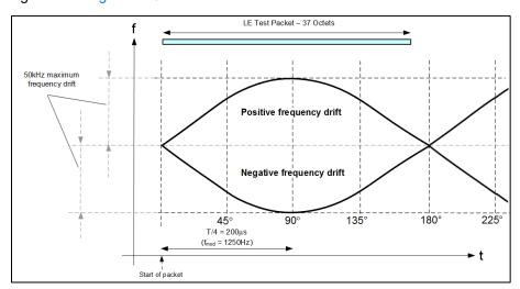
Figure 4.20: Dirty transmitter frequency drift emulation principle
