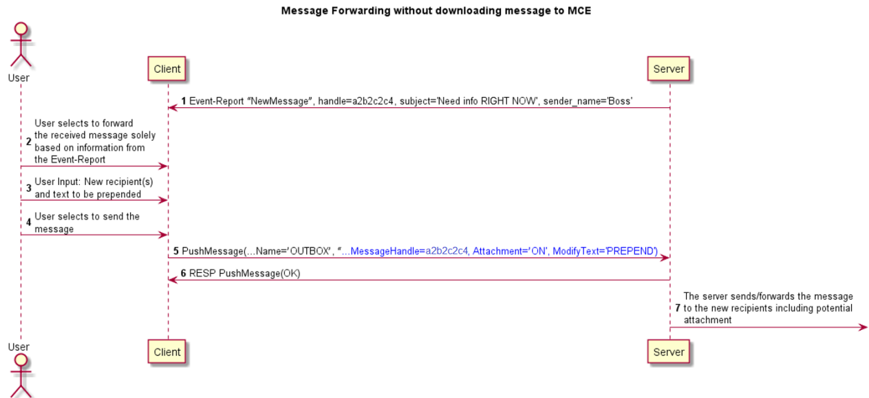
Figure 4.12: Example sequence for forwarding a message without downloading the message to the MCE
