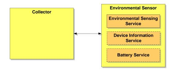
Notes: Profile roles (Collector, Environmental Sensor) are represented by yellow boxes and services (Environmental Sensing Service, Device Information Service, and Battery Service) are represented by orange boxes.
